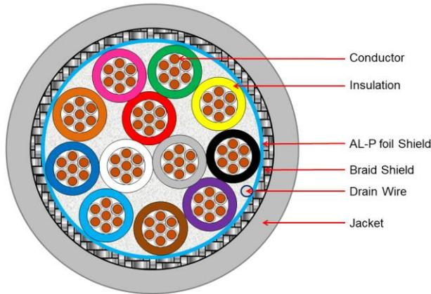
LINK Multi-Core cable, 12 cores Double Shield
