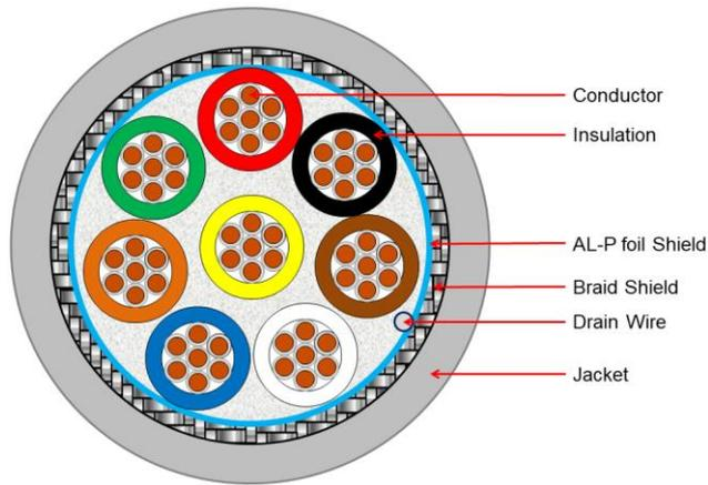
LINK Multi-Core cable, 8 cores Double Shield
