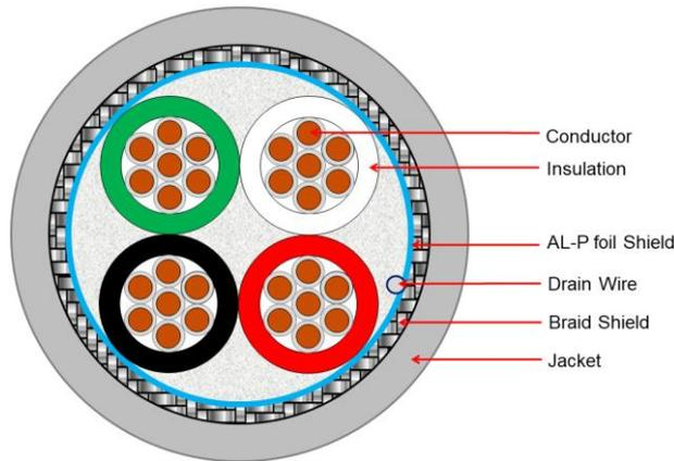
LINK Multi-Core cable, 4 cores Double Shield
